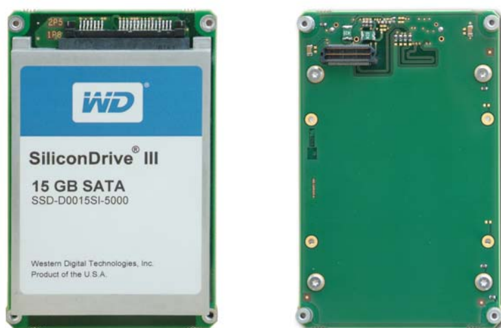
Figure 27: SATA Extension Module: Front and Bottom Views
