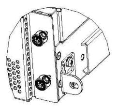
**Universal Front Mounting Bracket with securing tab**
